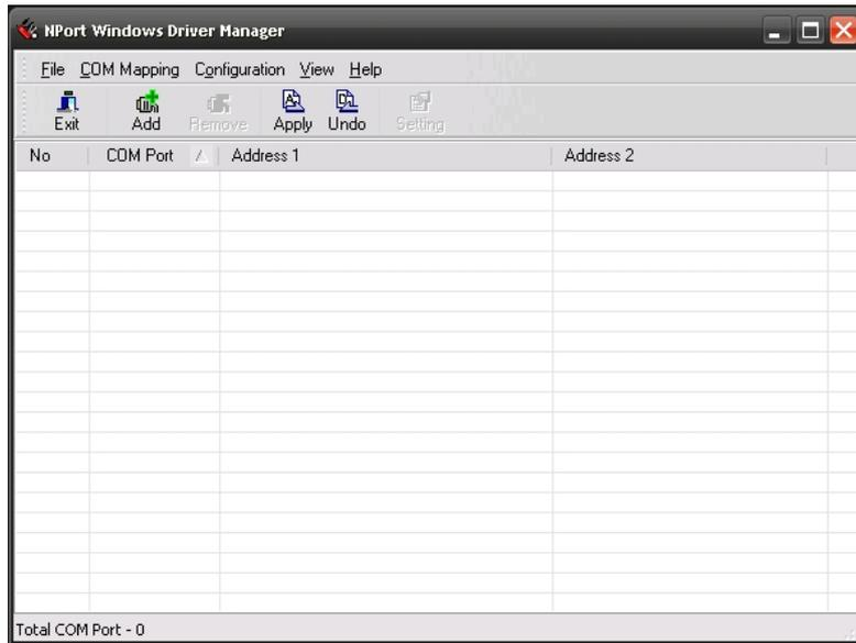
Figure 1.16: Moxa NPort Driver, Add device/ports
