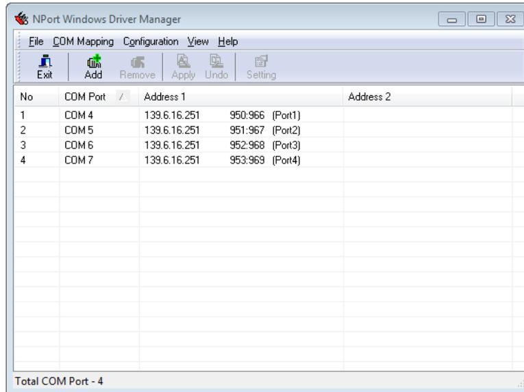
Figure 1.18: Moxa NPort Driver, COM Port Mapping
