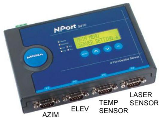
Figure 1.15: Moxa NPort 5410 Serial Device Server
