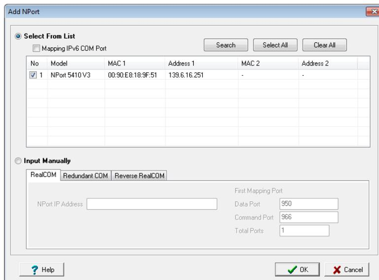
Figure 1.17: Moxa NPort Driver, Search Devices on the Network
