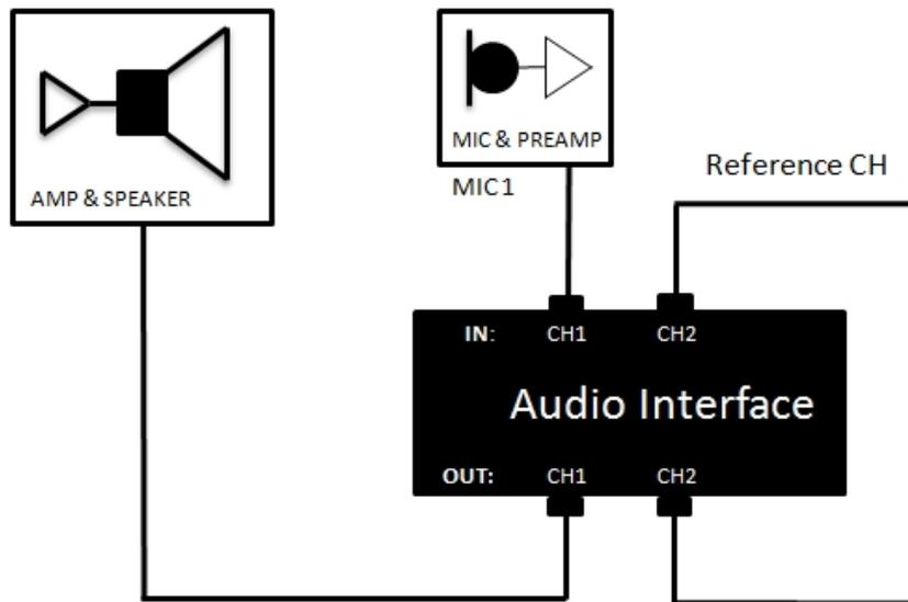
Figure 1.21: Audio cabling for using the Windows default audio device
