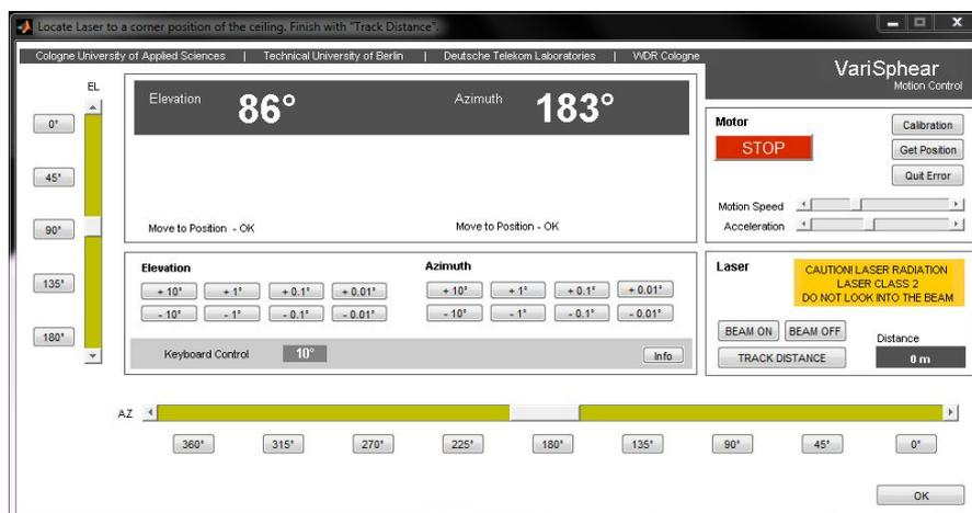
Figure 3.2: VariSphear rCg coordinate acquisition
