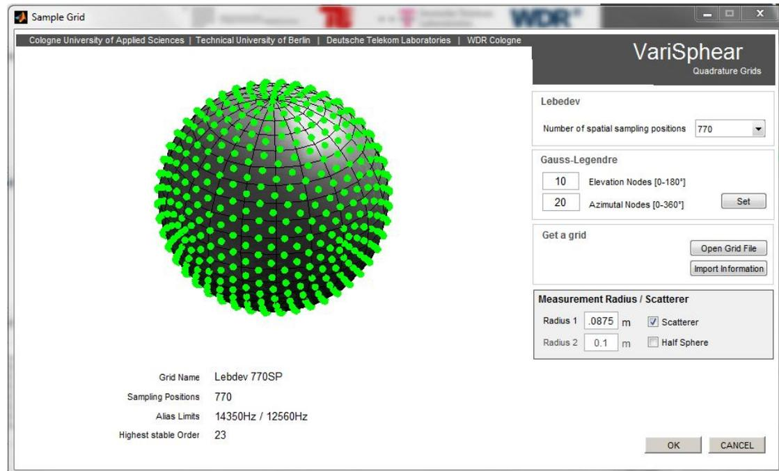
Figure 2.3: VariSphear Select Sample Grid
