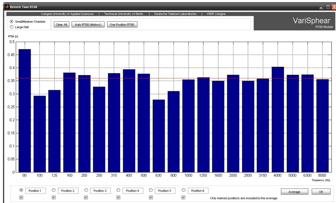
Figure 2.6: VariSphear RT60 Module
