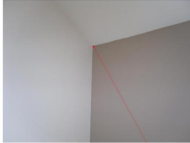
Figure 3.3: Locating a ceiling corner with the laser unit
