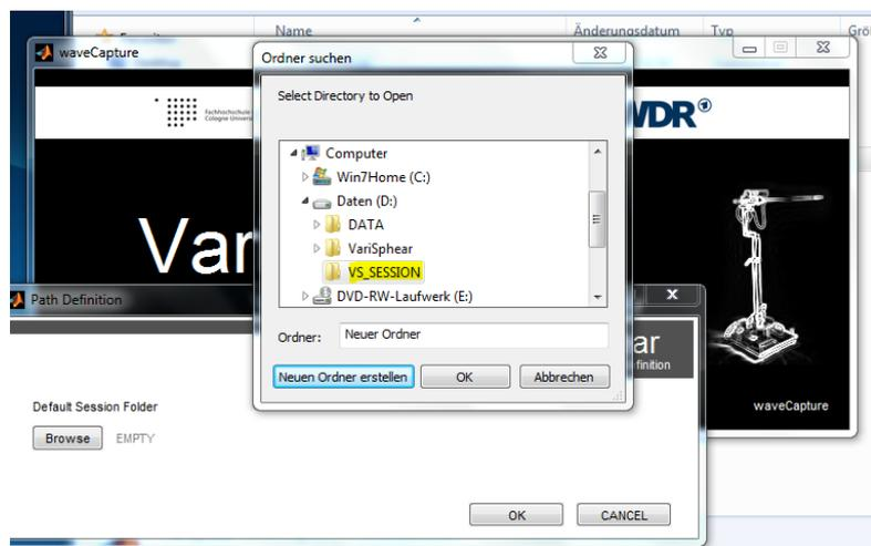
Figure 1.12: STEP 9: Create a new folder for the session path or use an existing session path from a previous VariSphear software.
