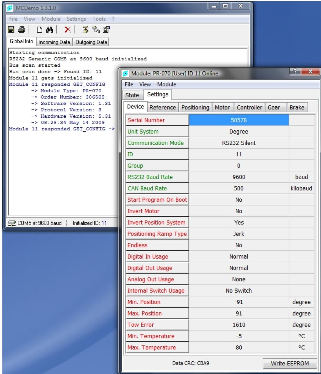
Figure 5.2: VariSphear ELEVATION Motor Configuration still in User-Mode
