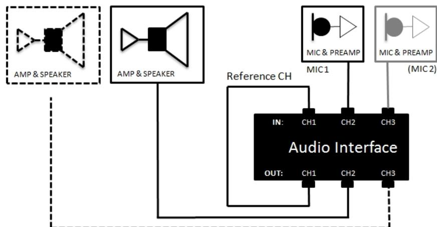
Figure 1.20: Example audio cabling for ASIO driver with reference and 1 or 2 Mics
