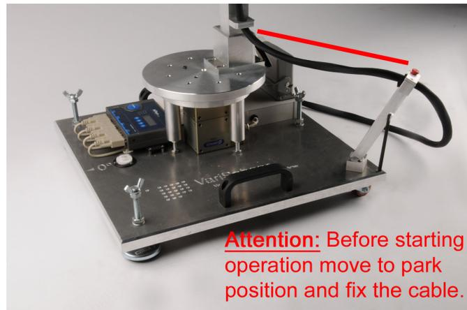
Figure 1.3: VariSphear - Remind to mount the cable in the correct position
